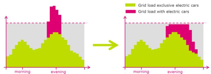
Figure 1: Uncontrolled charging vs. smart charging
