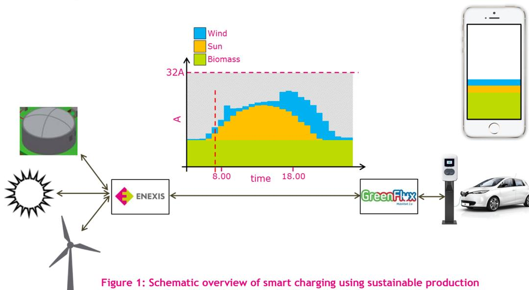
Figure 1: Schematic overview of smart charging using sustainable production
